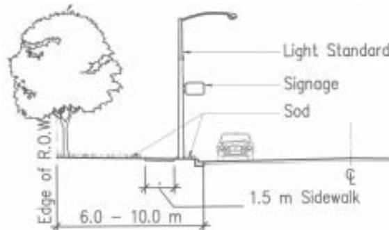
Figure 4.1.1h - Existing Road Edge Condition 4 Sidewalk with no Splash Strip
