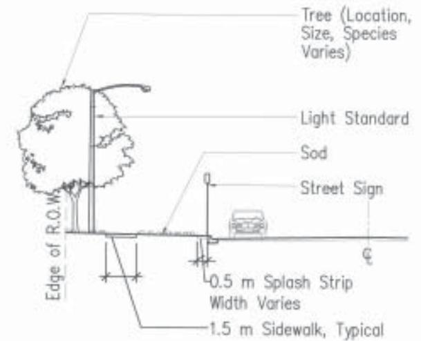
Figure 4.1.2 b - Existing Road Edge Condition 5 Sod Strip Between Sidewalk & Splash Strip
