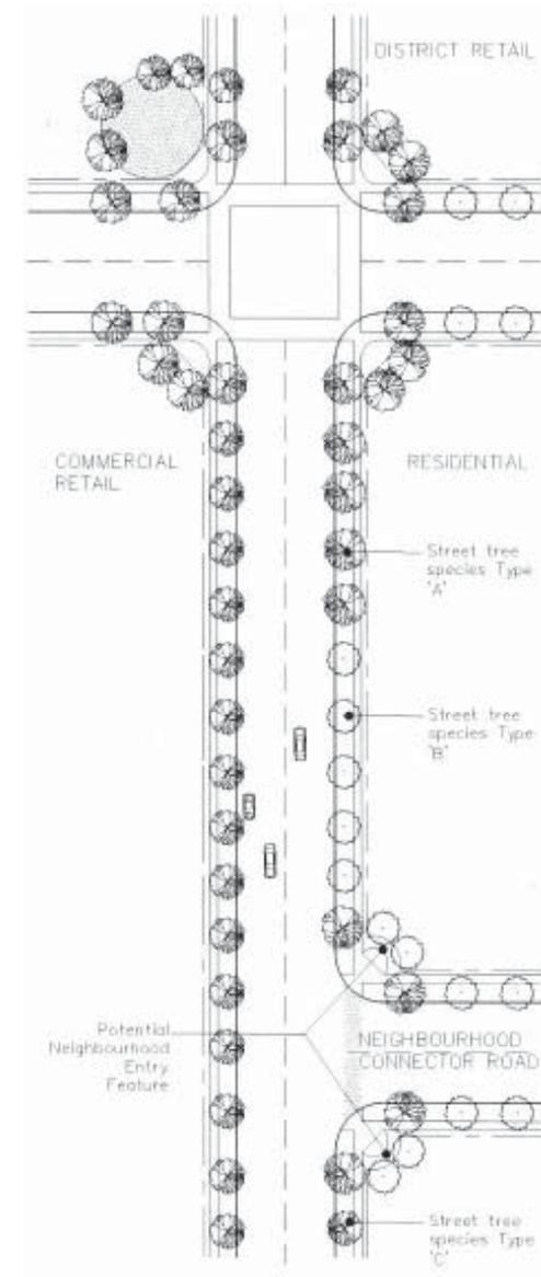
Figure 2.2c Schematic Plan of Tree-Lined Arterial Road
