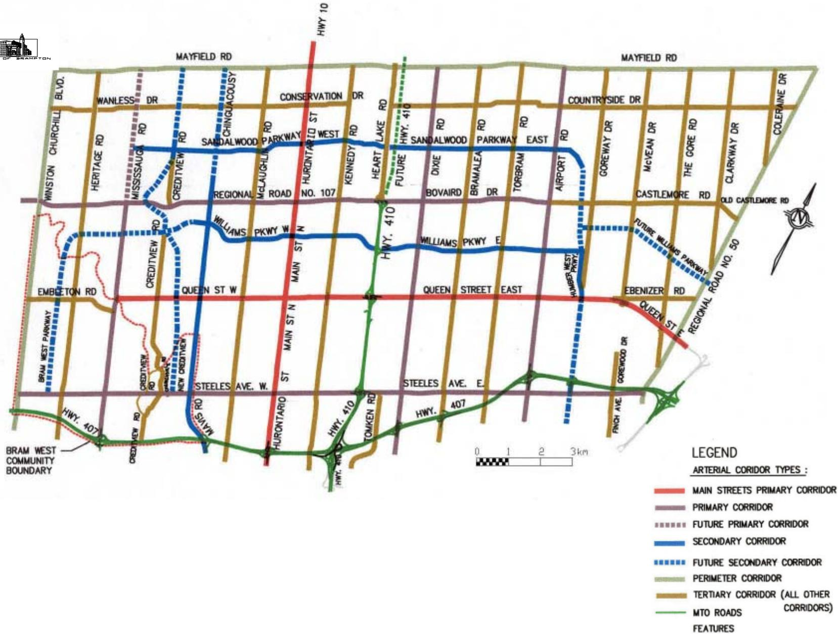
Figure B.1 - Arterial Corridor Hierarchy Mapping
