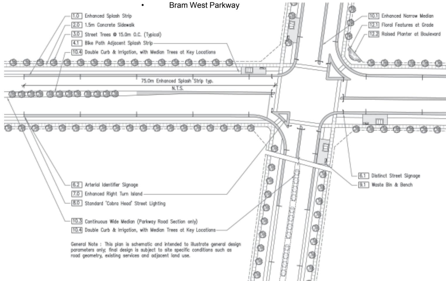
Figure 5.2.3 Enhancements for Secondary Arterial Roads.
