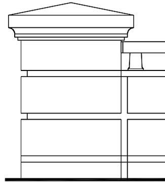
Figure 5.4.1a Bridge End Pier Elevation
