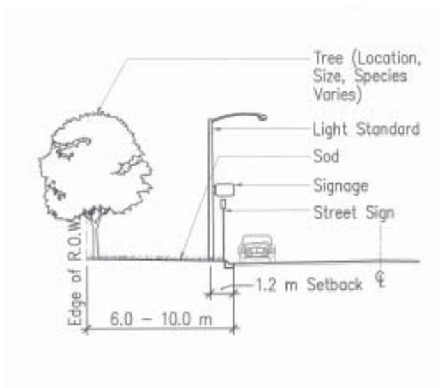
Figure 4.1.1.e Existing Road Edge Condition 3 No Sidewalk
