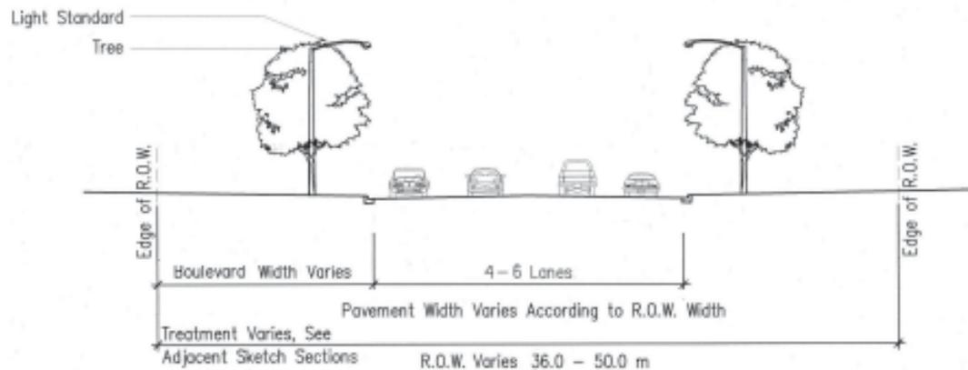
Figure 4.1.1 a - Existing Arterial Prototype Section at Built-up Areas
