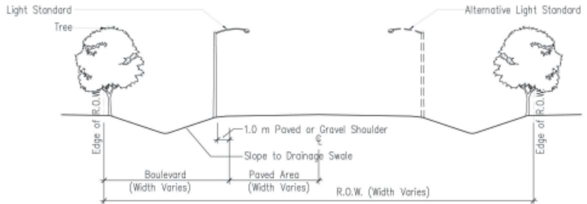
Figure 4.1.1 i - Existing Arterial Prototype (Rural Road Section)
