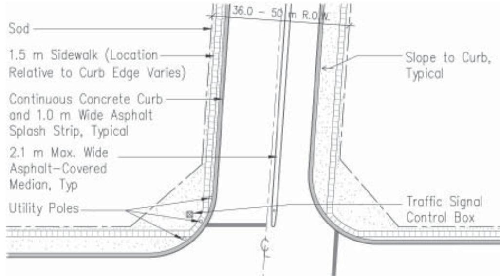
Figure 4.1.1 d - Plan of Arterial Intersection at Developed Areas
