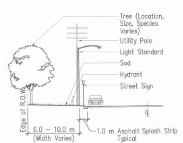
Figure 4.1.1 b - Existing Road Edge Condition 1 No Sidewalk
