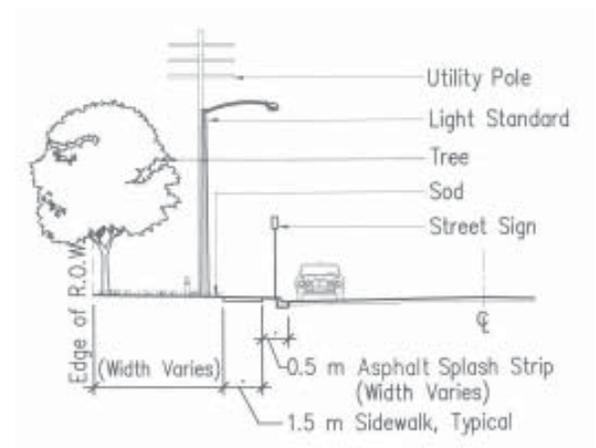
Figure 4.1.1 c - Existing Road Edge Condition 2 Sidewalk Adjacent Splash Strip
