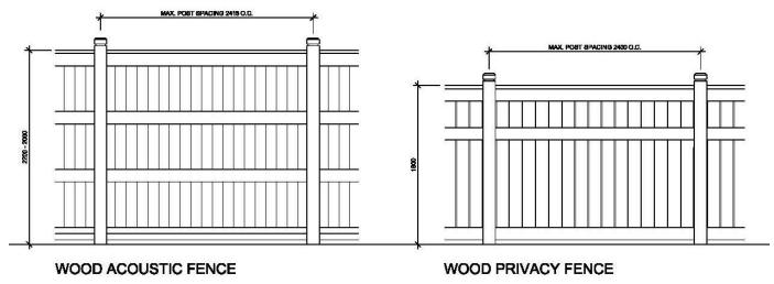
Figure 46b - Fencing Conceptual Design
