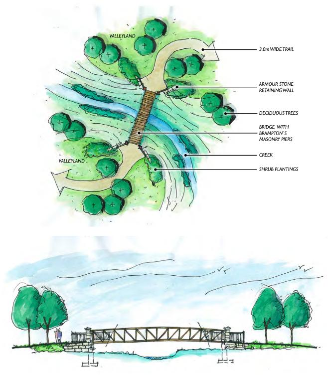
Figure 35 - Example of Pedestrian Bridge as per City of Brampton's Standards
