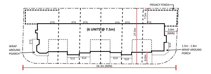
Figure 49 - Cap-End Townhouse Block with 7.5m Units
