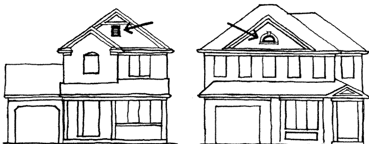
Figure 7 Avoid Black Glass in Roof Elements
