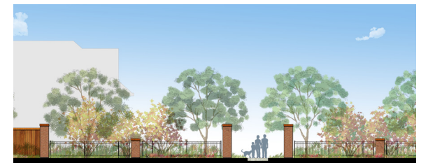
Fig. 3.1.2.4b - Conceptual elevation of a typical window street design with masonry or stone columns, ornamental metal fence and higher planting density.
