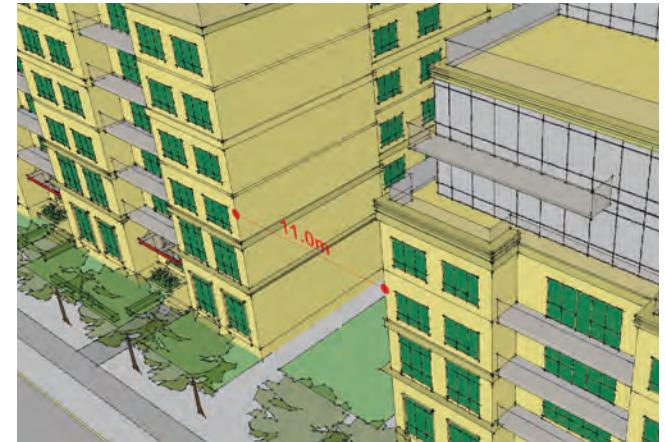
Figure 6-59: Spatial separation between buildings
