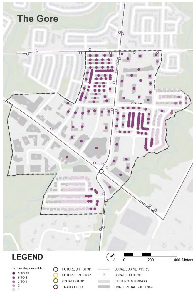
Figure 6-192: Access to local bus service at a 400 m walking distance within The Gore MTSA
