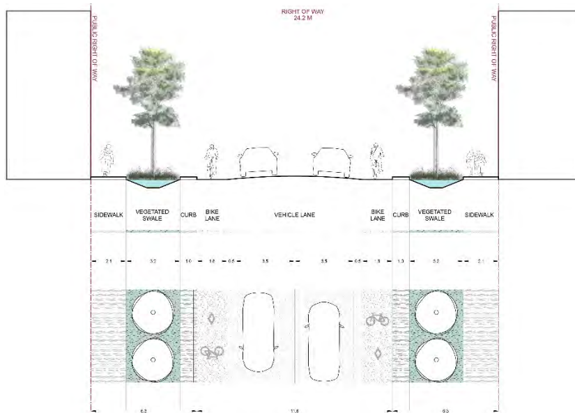
Figure 5-11: Optimized Local Employment Complete Street Cross-Section
