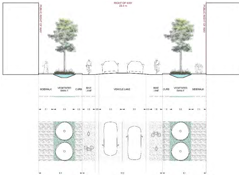
Figure 5-7: Optimized Downtown Complete Street Cross-Section
