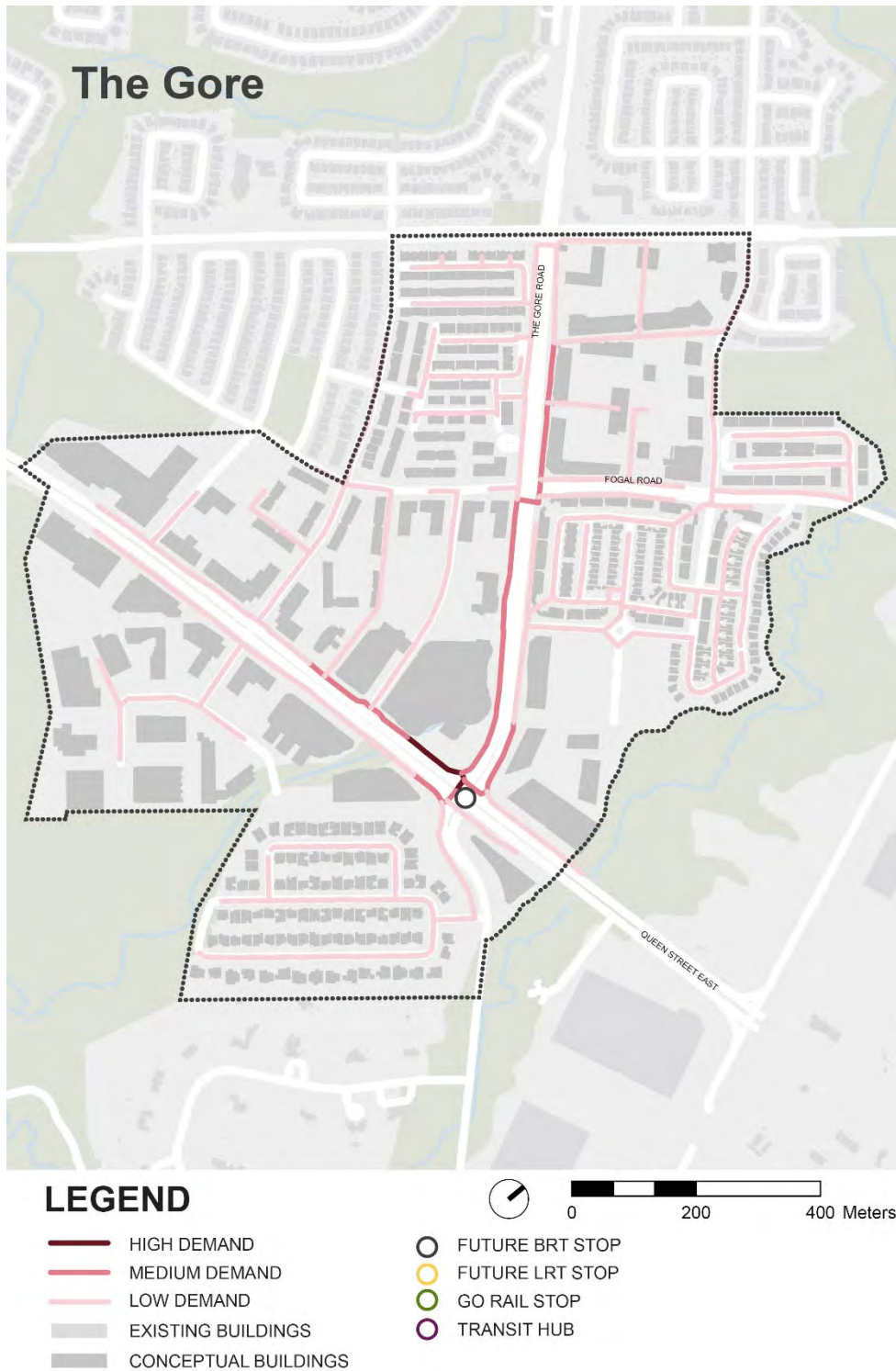
Figure 6-191: The Gore Aggregation of Walk Demand to and from the Nearest Transit Stop
