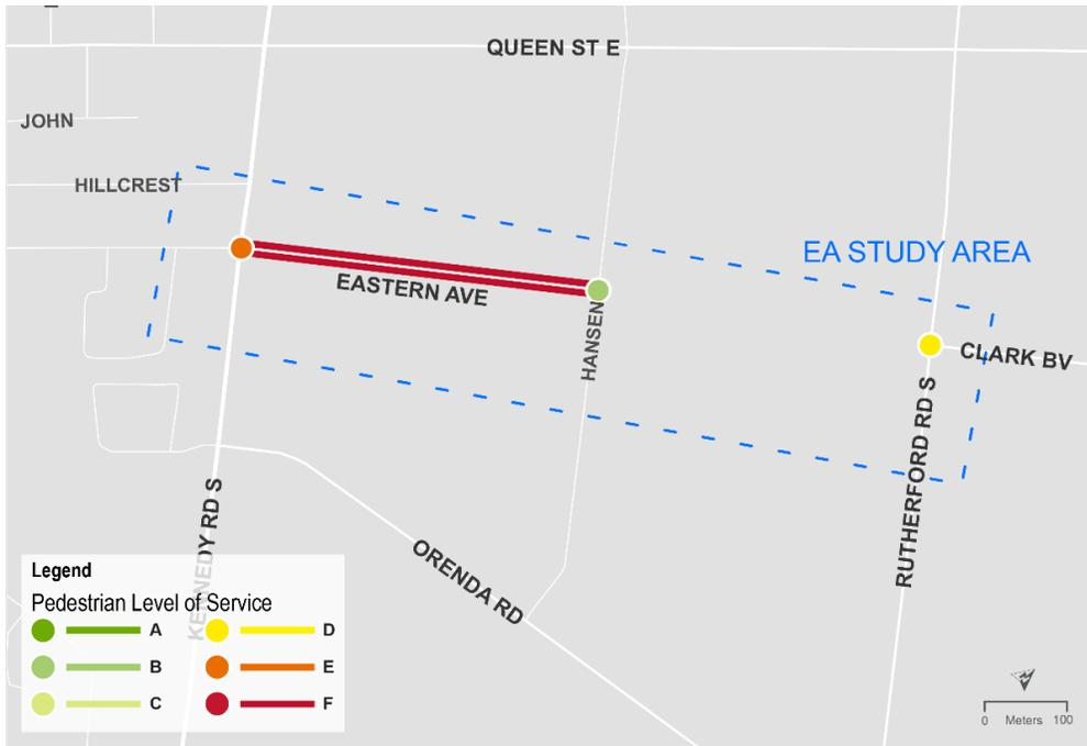
Figure 3-7: Pedestrian Level of Service (PLOS)
