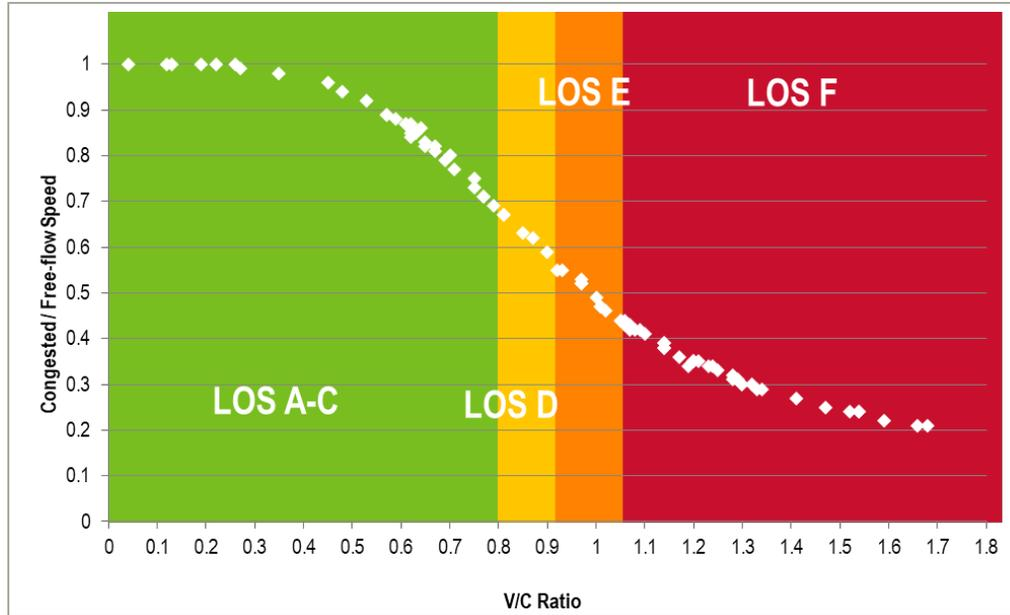
Figure 2-1: Relationship between Congested/Posted Speed Ratio and V/C Ratio
