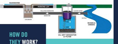
Oil and other pollutants collect on paved parking lots, driveways and roads over time and then are washed off by stormwater and into an Oil Grit Separator or filter.
