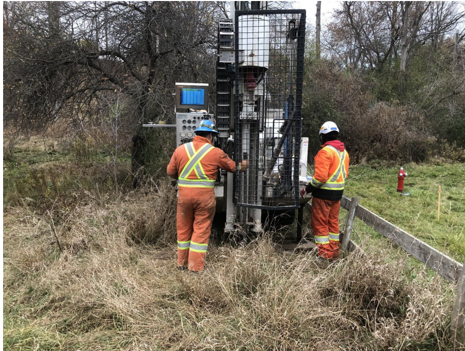
Photo 3-2: CPTu drill rig set-up at Churchville flood dyke (northern section on Churchville Road)
