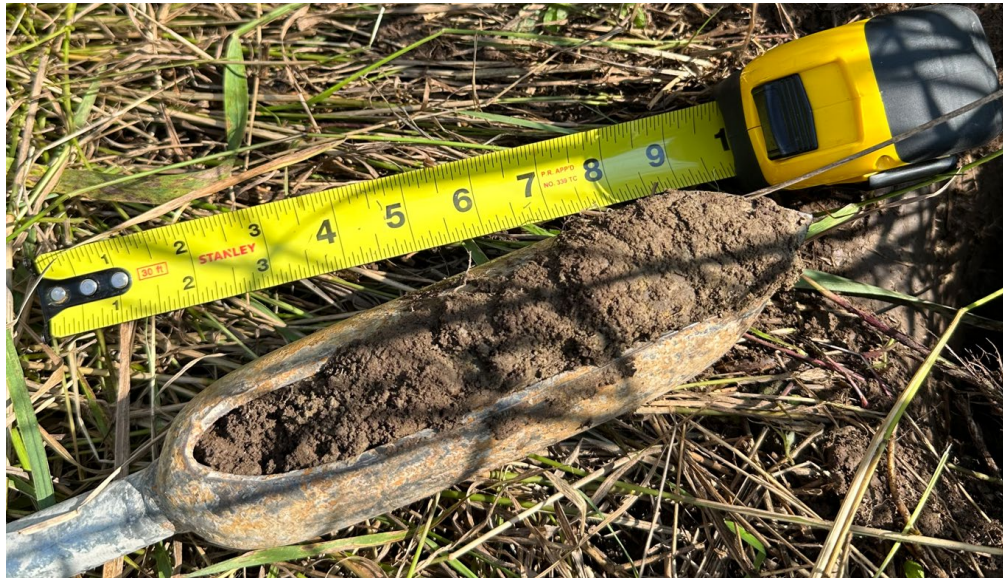
Photo 4-1: Typical dyke fill recovered during geotechnical investigation
